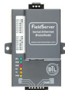
IS to Bacnet / Lonworks
